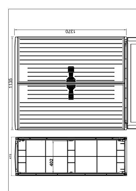
tested according to VDE 0660 part 500 / IEC 439-1 usable internal depth of 402mm at the closing TÜV according to DIN EN 61439-5 Special depth 470mm
